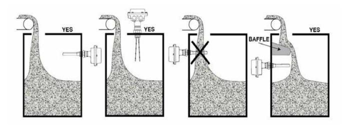
If the fork is mounted horizontally, it must be positioned so that the material will not accumulate on top of the tines. There is an index mark on the mounting nut to assist in proper positioning of the fork.
