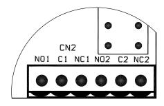
Figure 8. Auxiliary Relay Connections - ADVANCED ONLY
