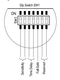
Figure 13: Switch Functions, Advanced
